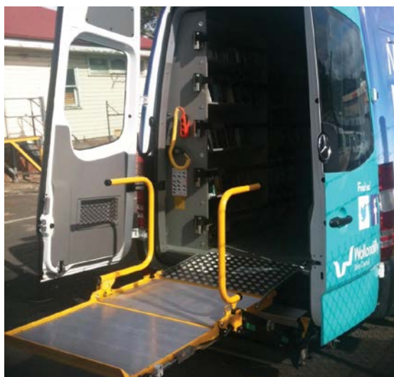
/WHEELCHAIR LIFT FITTED TO REAR OF THE MOBILE
