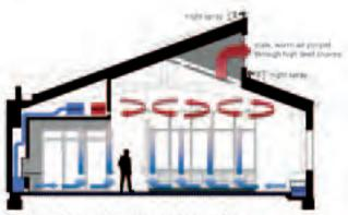
Figure 5. Summer Cooking, Hydronic Stats and Air Conditioning System.
