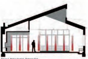
Figure 6. Winter Heating, Hydronic Stab Warreth is radiated from the Room stab by pinculating earns exist inmosph populated into the stab. This eater is heated using the feat juring system.
