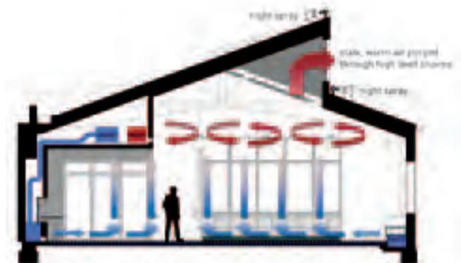
**Figure 5. Summer Cooling, Hydronic Slab and Air Conditioning System**
