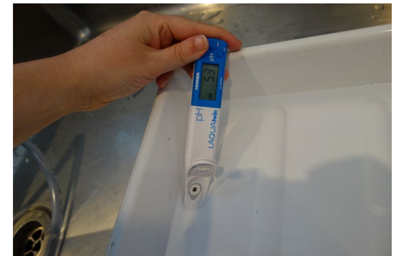
Measuring pH value of a wash bath with the Laqua meter
